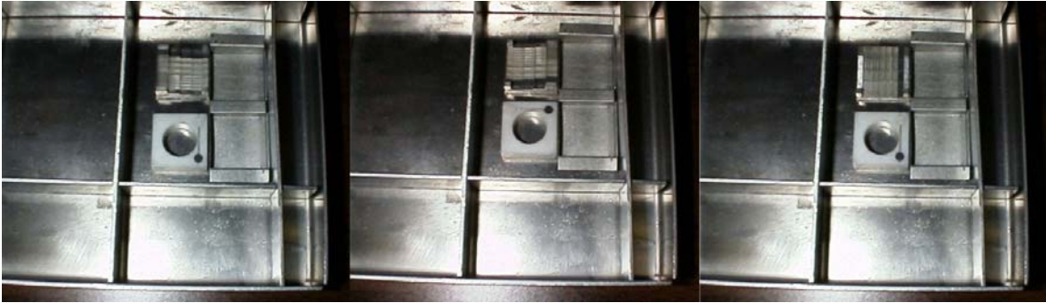
Figure 17.5: Incorrect placement of indicators in part holder (three examples)
