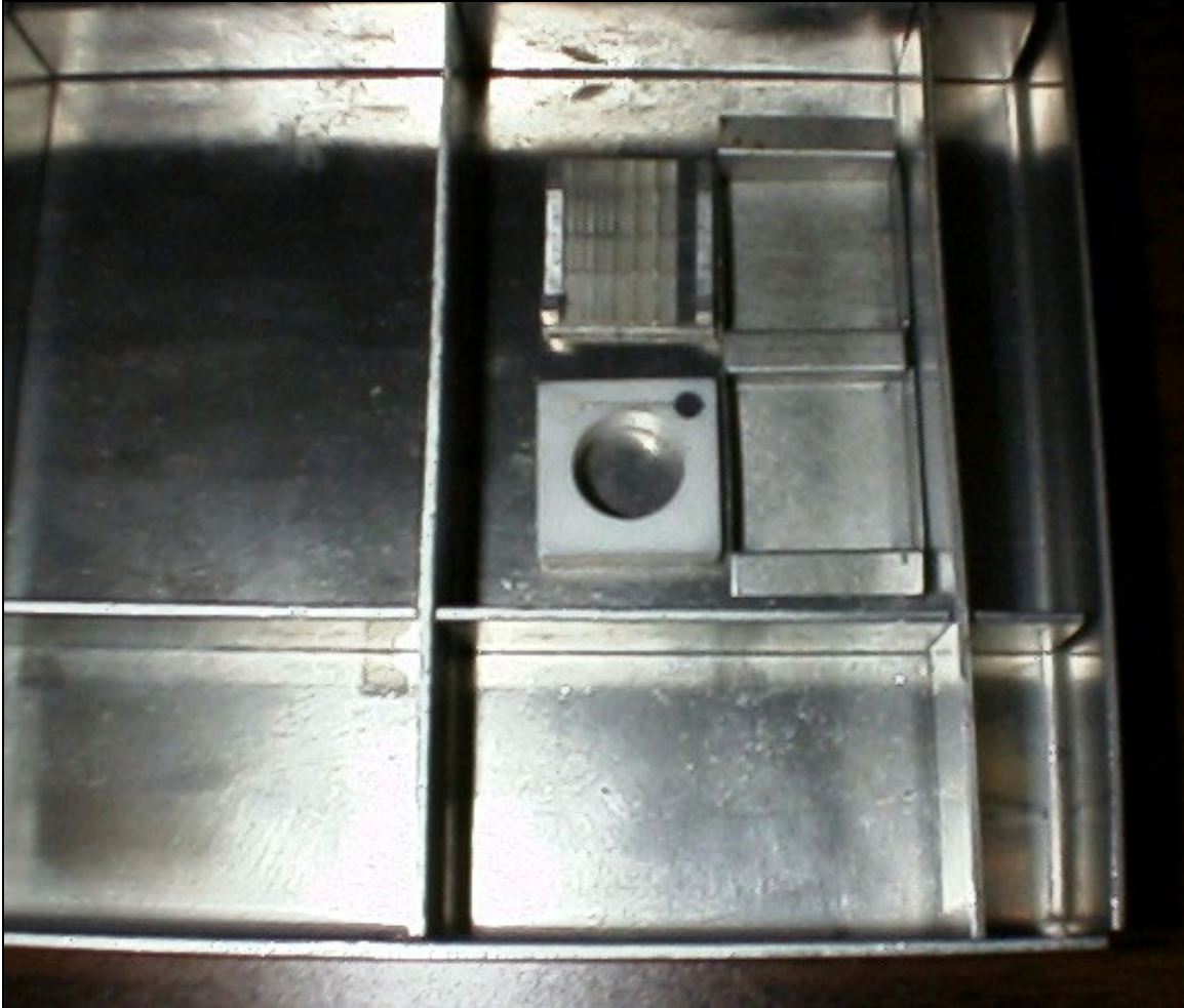
Figure 17.4: Correct placement of Indicators in part holder
